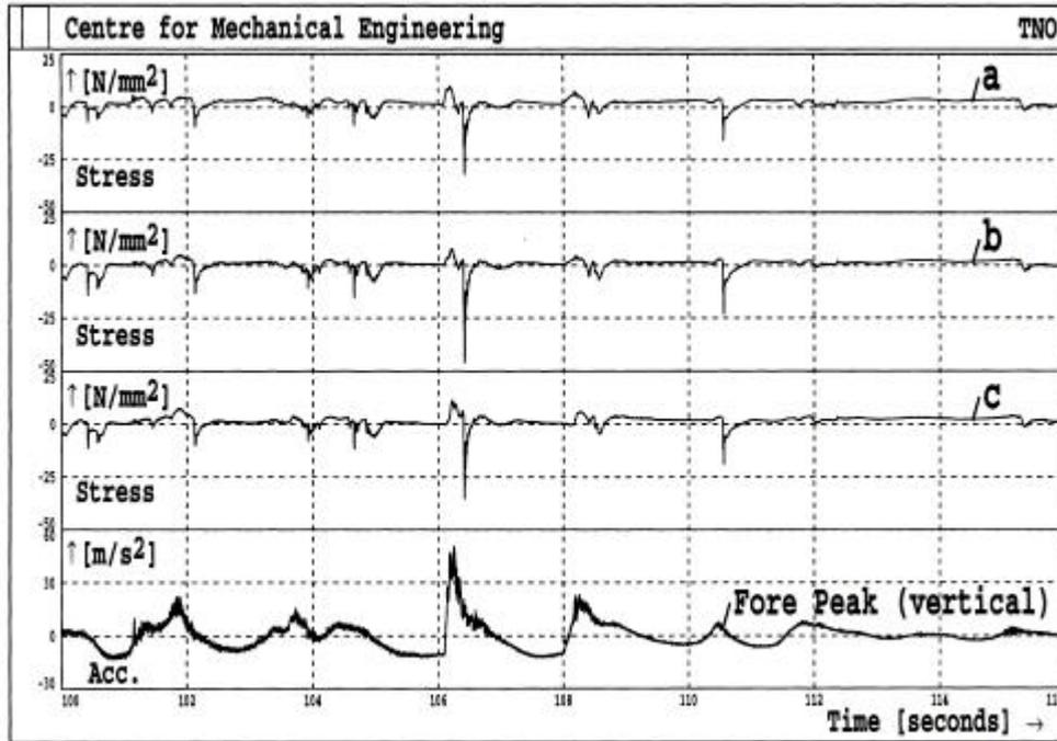
Figure 9 Hull Stress Level Measurement Results for Frame 10 at 2<sup>nd</sup> Spray Rail PS, in Sailing Condition BF 8, Significant Wave Height 2.5 Metres
