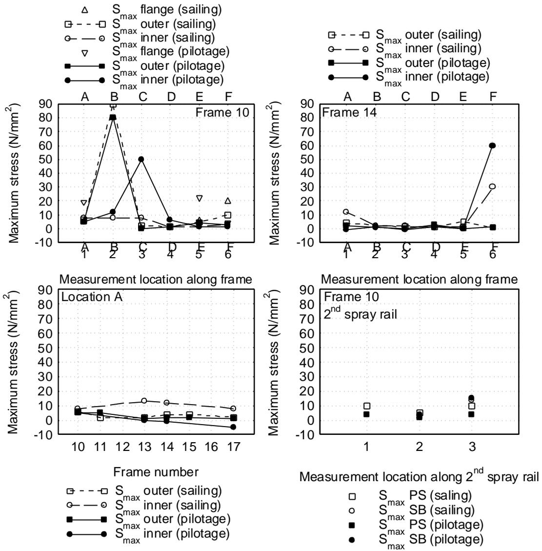
Figure 8 Hull stress levels during pilotage and sailing conditions
