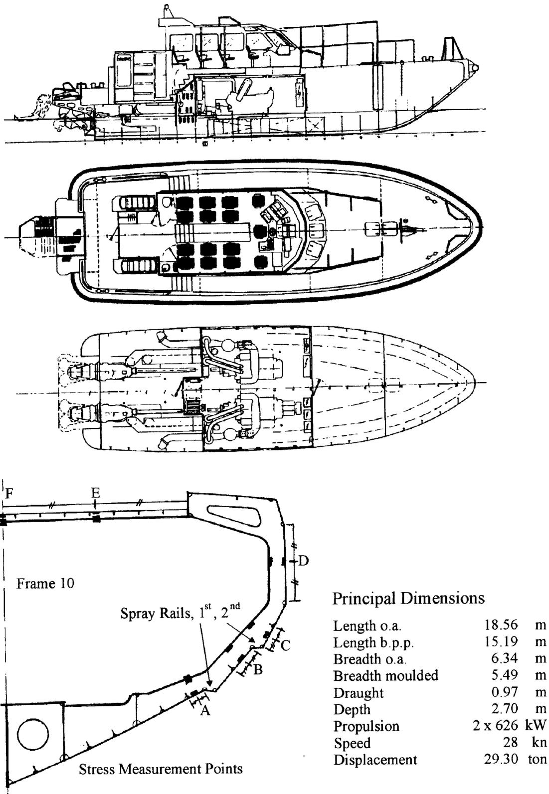
Figure 1 General Arrangement MS VOYAGER and Frame Section Number 10
