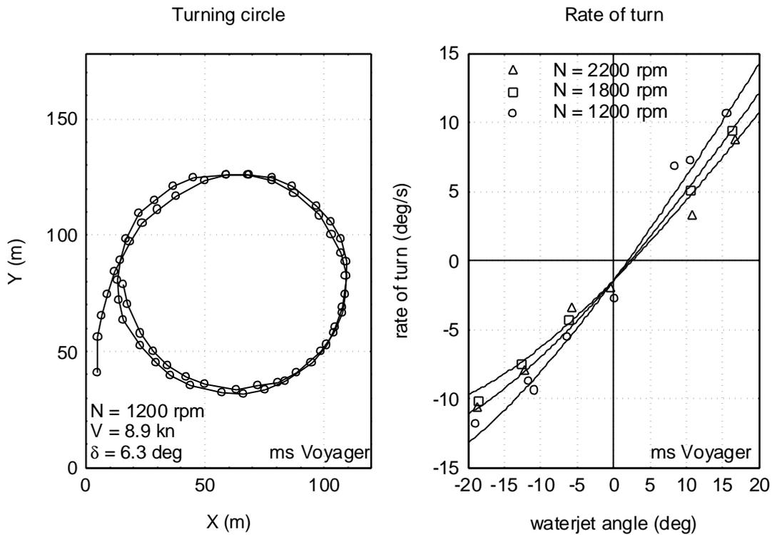
Figure 4 Manoeuvring tests in calm water
