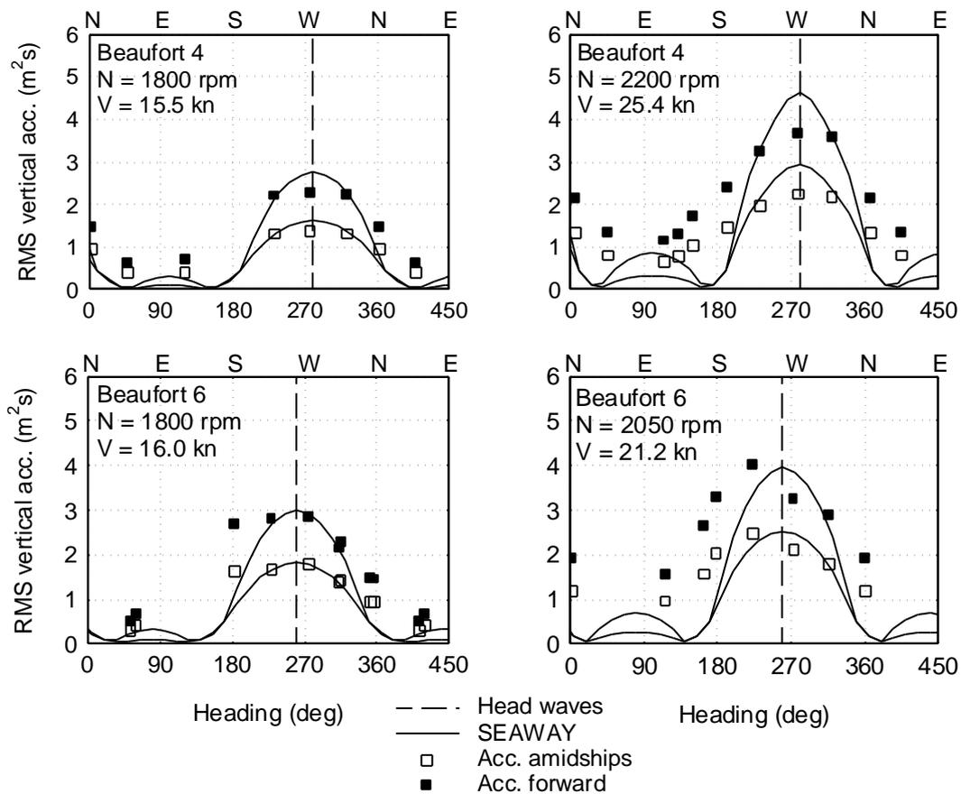
Figure 5 Measured and computed RMS values of vertical accelerations
