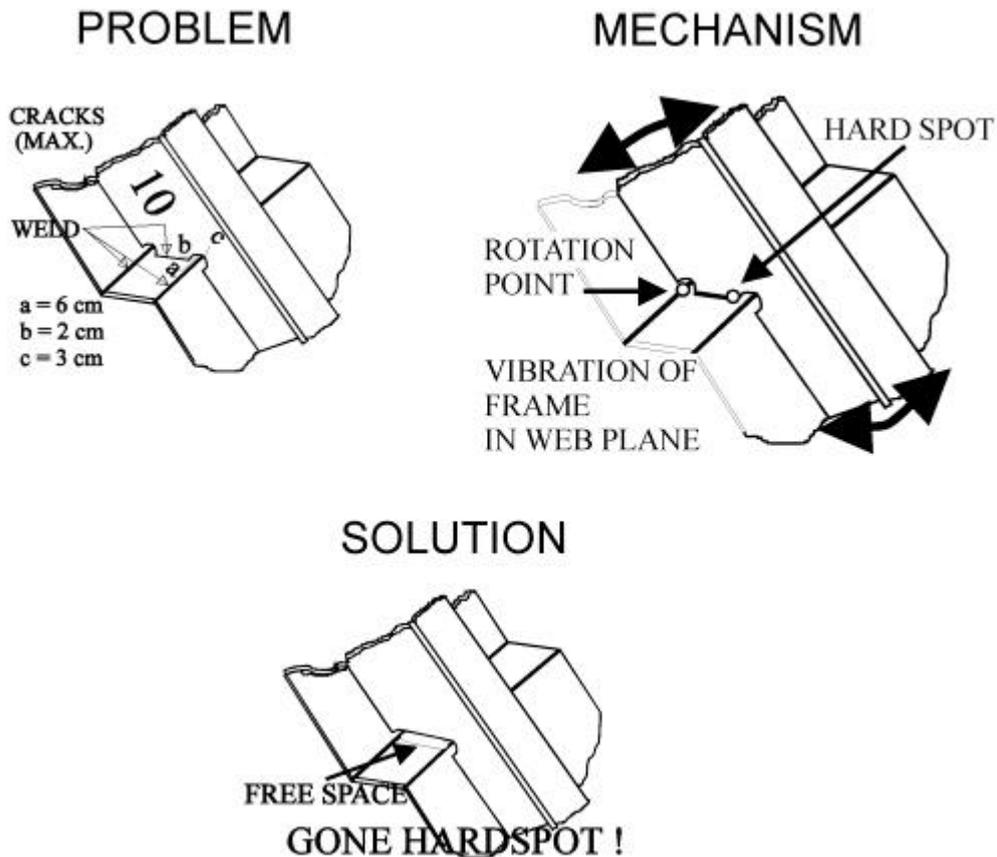
Figure 10 Structural Improvement 2<sup>nd</sup> Spray Rail
