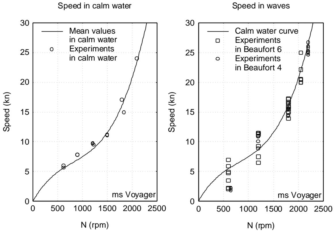
Figure 2 Speed Trials in Calm Water and in Waves
