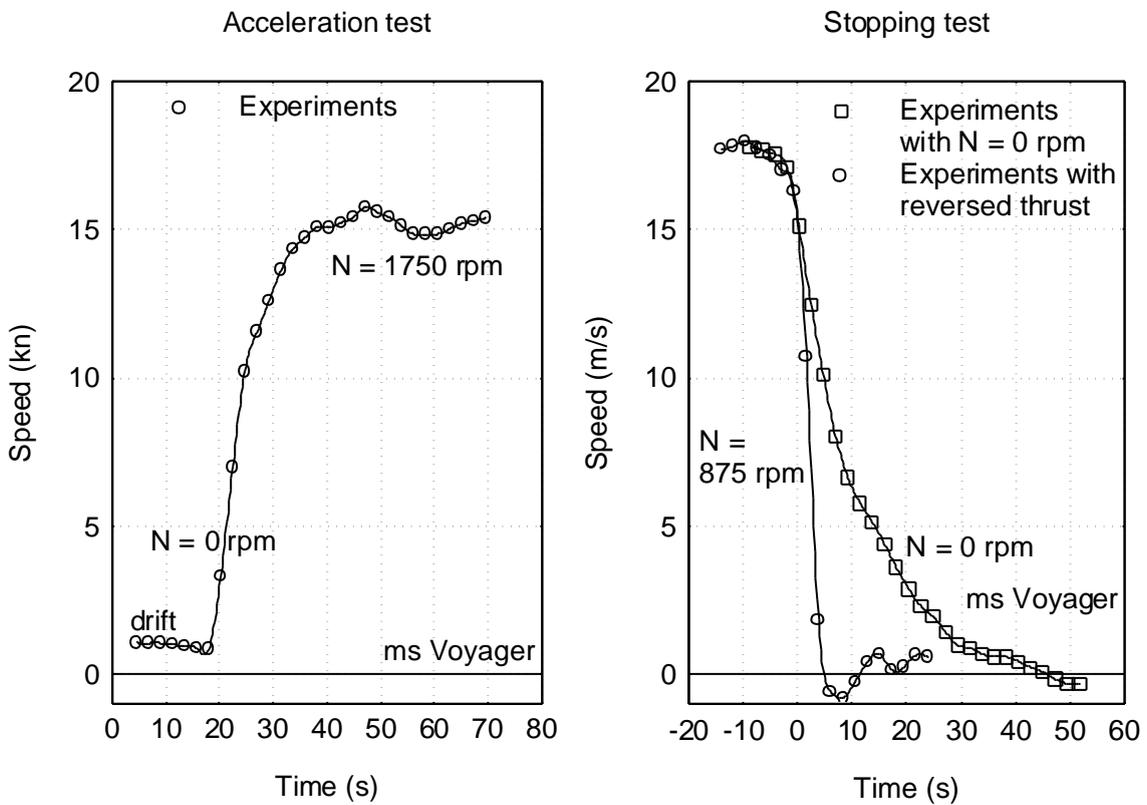
Figure 3 Acceleration and Stopping Tests in Calm Water
