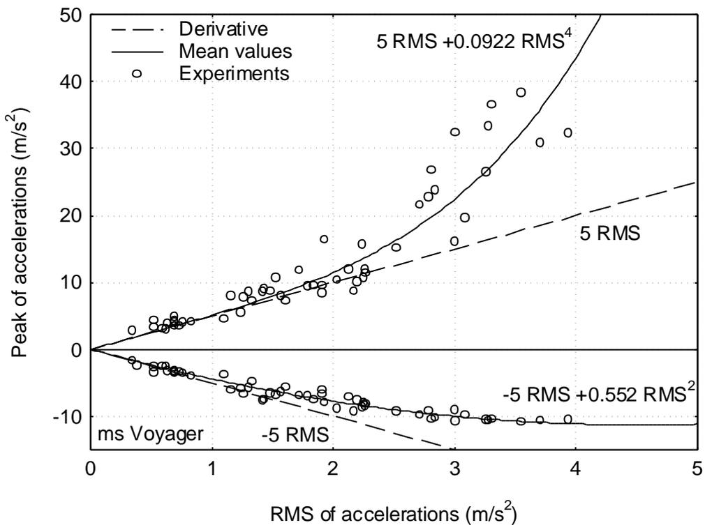
Figure 7 Peak versus RMS values of vertical accelerations forward}
