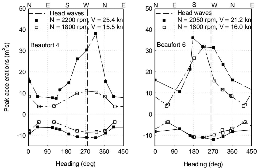
Figure 6 Measured peak values of vertical accelerations forward}
