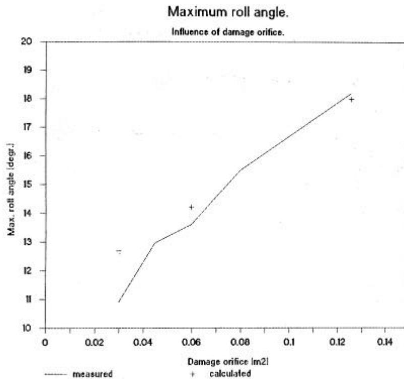
Figure 9 Maximum Roll Angle Versus Area of Damage Orifice
