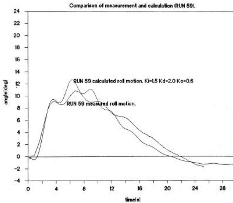
Figure 7 Roll Motion Run 59 (Damaged Orifice Decreased)
