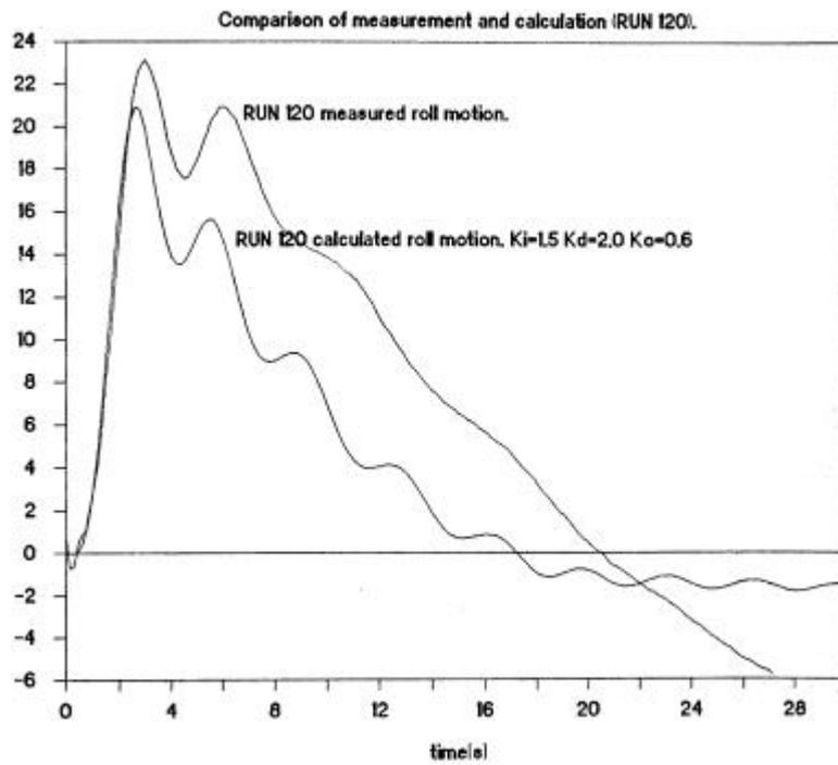
Figure 8 Roll Motion Run 120 (Height of CoG Increased)
