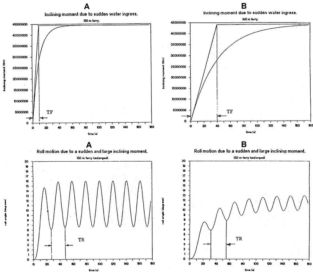
**Figure 1 Rough Estimates of Roll response to Sudden Water Ingress**
