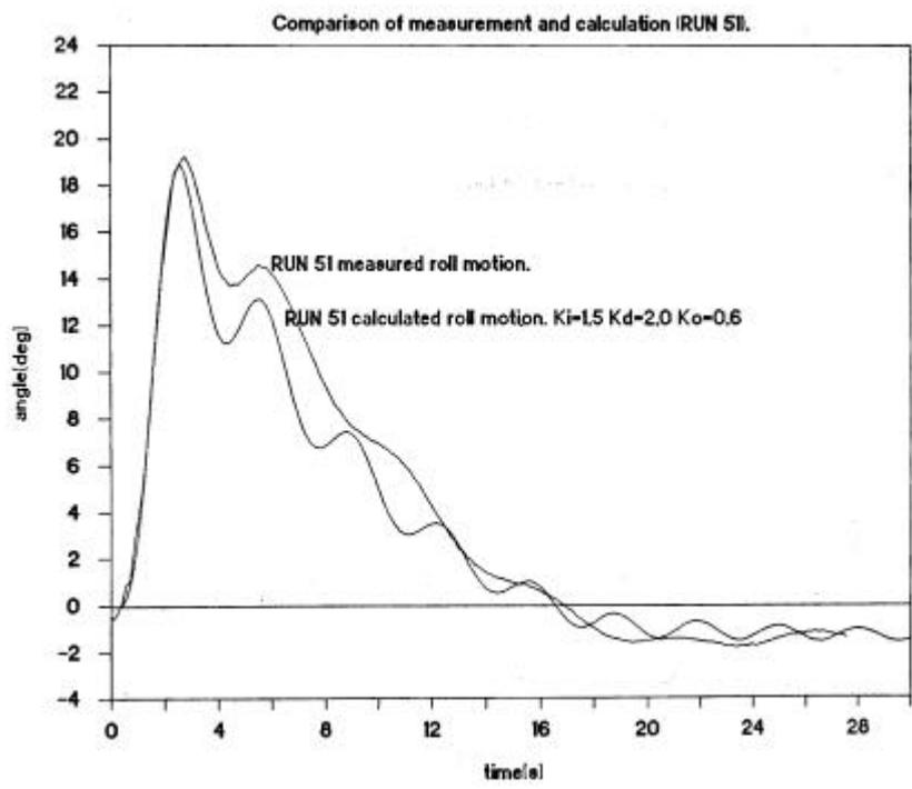
Figure 5 Roll Motion Run 51 (Area of Vent. Holes Increased)
