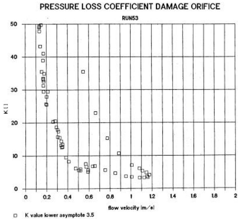
**Figure 10 Pressure Loss Coefficient as Function of Flow Velocity, Damage Orifice**
