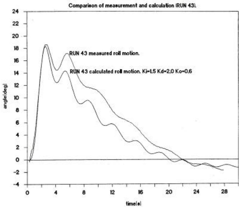
Figure 4 Roll Motion Run 43 (Decreased Duct Area)
