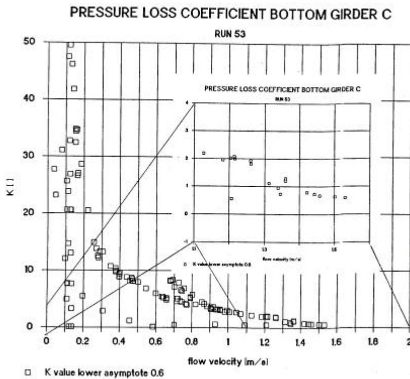
**Figure 11 Pressure Loss Coefficient as Function of Flow Velocity, Orifice C**
